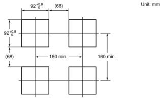
Normal Allowable Deviation= $\pm$ (Value of JIS B 0401-1999 tolerance grade IT18) / 2
